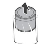
3. Remove the protective vinyl from the filter installed inside the product.
