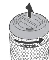
2. Grab the handle at the bottom of the product, turn counter-clockwise, and pull out the filter cover.
