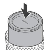
4. Install the filter top side down into the bottom of unit until it is fully inserted. The top of the filter shows the opening and the bottom of the filter is solid.
