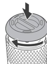
5. After installing the filter, turn the handle clockwise to close the filter cover.
